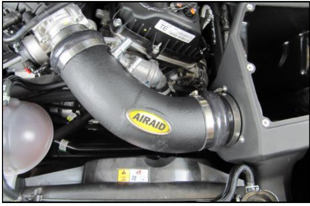
10. Insert the Intake Tube into the Hump Hose and Reducer then tighten all 4 Intake Clamps.
