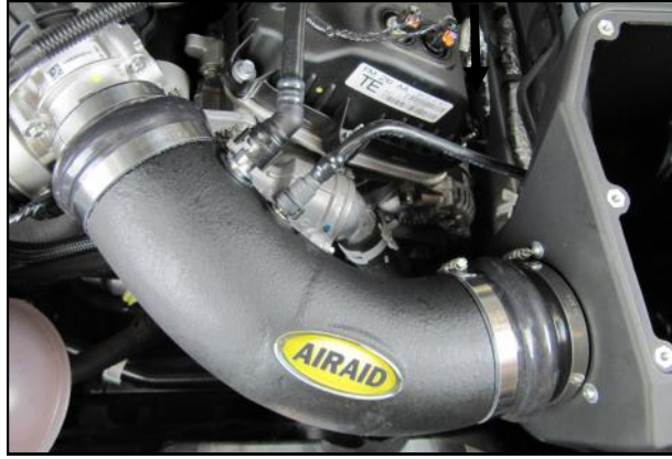
11. Reconnect the breather hoses to the Fittings in the Airaid Intake Tube.
