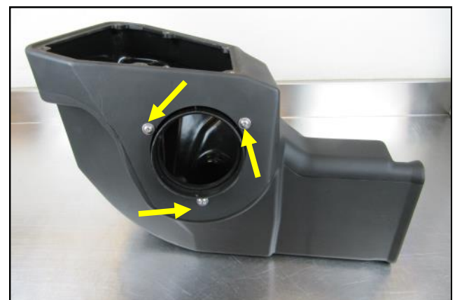
6. Install the Filter Adapter onto the Cold Air Box as shown, using three sets of 1/4-20 Button Head Screws and 1/4" Flat Washers
