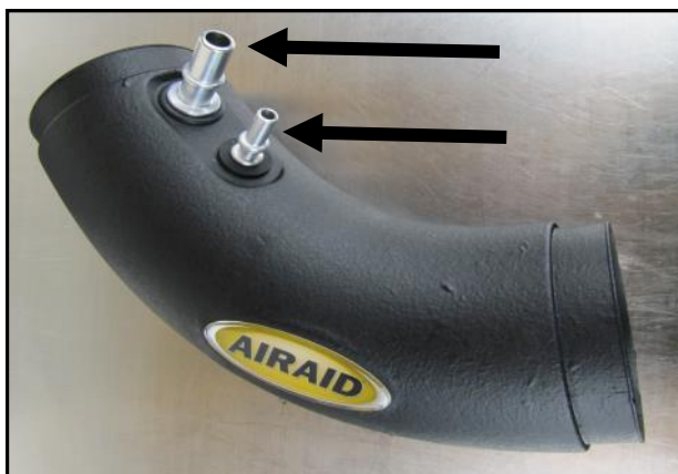
5. Install the Grommets and Aluminum Fittings into the Airaid Intake Tube. Apply the Airaid Decal as shown.
