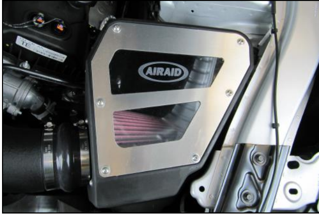
13. Remove the protective film from the Lid and Window before installation. Install the Airbox lid and Window onto the Airbox, with the Window on top, using 6 sets of 1/4" Button Heads, and Washers, and Washers.
